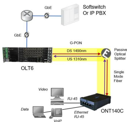
Though not as common, the OLTs and ONTs can also support analog voice, or what is commonly called Plain Old Telephone Service (POTS). In this scenario, the ONT itself contains a Session Initiation Protocol (SIP) to the analog converter that allows the POTS phone to plug into an RJ-11 port on the ONT. As the ONT converts the POTS call to SIP, it is transported over the Optical LAN system in a VoIP format.
