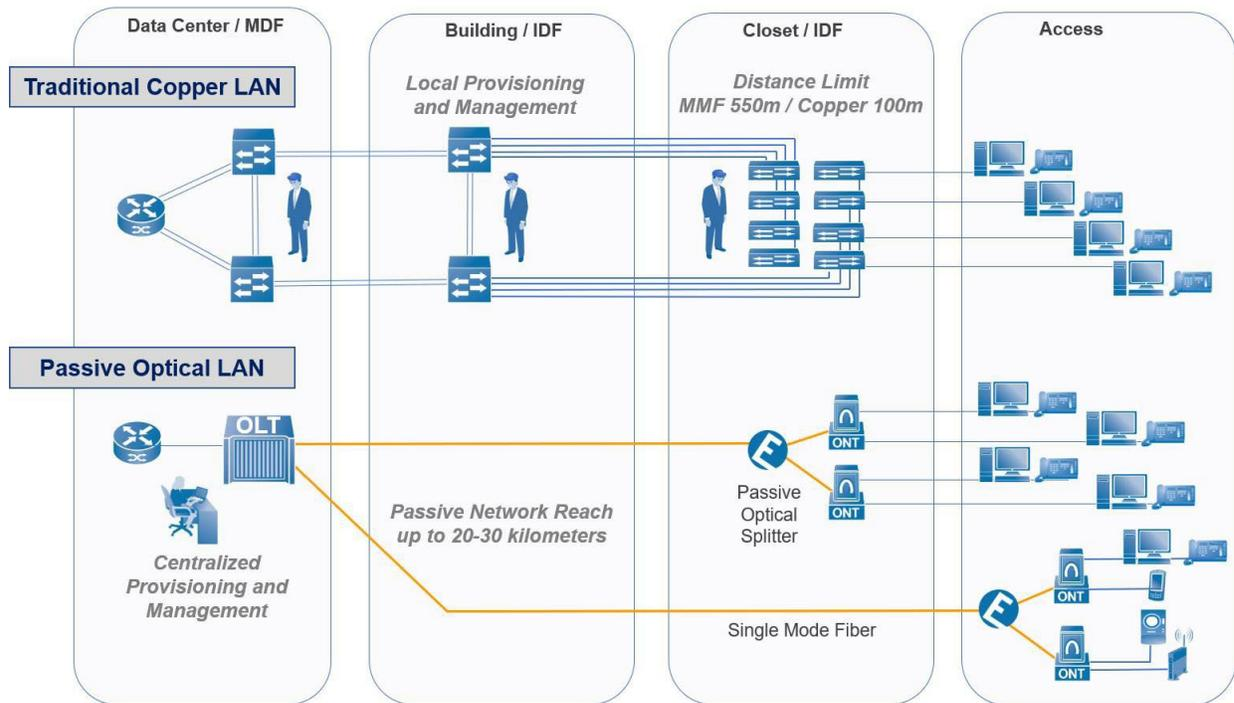
**Legacy Copper LAN** – In a traditional copper-based LAN, a router in the top-most layer (Core Layer) links to the campus or building aggregation switches (Distribution Layer). The distribution switches connect down to the Access Layer switches in the communications closets. Copper cables extend from the communications closets to the users and end devices.
